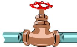
City Code requires that each water connection have a hand valve on the owner’s side of the meter.
